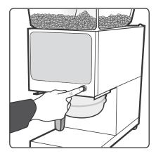
5 Push the START button on the front panel. The grinder will start to grind coffee into the brew basket. It will stop at the set volume.
